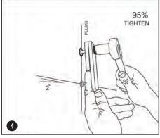
**4. BOTH:** Slide a washer onto a 75mm bolt and slide this through the top holes of the entire 'MTA' (1-hole tab under 2-hole tab) now tighten into the top drilled hole with spanner to 95% tightness.
