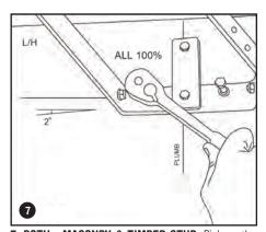
**7. BOTH - MASONRY & TIMBER STUD:** Pick up the clothesline bracket and slide under the 'MTA'. Hand screw remaining 3 x M8 316 coach bolts & washers through bracket into wall plugs or timber to 100% then nip up the top bolt to 100%. The bracket should tilt 2° inward toward the next bracket.
