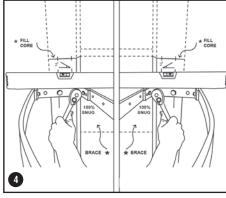
**4. INSTALLING 2ND BRACKET:** For location- feed cable through L/H bracket's 1st hole closest to wall pulling along wall & mark at the end of the cable. This is the centre hole location maximum distance of the R/H bracket. Repeat fixing process as per L/H bracket and tighten all bolts to 100% with 2° off set in place.
