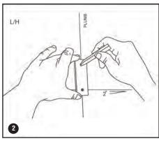
**2. BOTH:** Timber Studs mark centre holes on the stud line OR Masonry DO NOT drill into mortar lines. In the 'MTA' use the 2-hole piece, placing it on the marked vertical position with the lower of the holes centered on the marked cross line & mark through the top hole on the wall.
