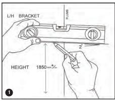
**1. BOTH:** Mark height location approx 185cm from ground level, use spirit level to draw a horizontal line for the bracket, slightly offset by 2° with an inward tilt (spirit level bubble will be uncentered). Draw a vertical line through the horizontal line marking both the centre hole bracket position. Use this method for ALL clotheslines.
