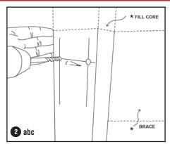
**2a. TIMBER POSTS:** Drill marked holes with 6mm drill bit to a depth of 75mm.
