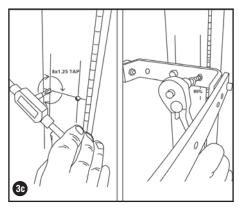
**3c. STEEL POSTS:** No Access Tap - Once drilled pick up M8 x 1.25 tap and lubricant. Slowly & methodically wind tap in with either a tap wrench or slow moving clutch drill winding in & out removing swaff. Once all holes are tapped place bracket onto post with hex bolts & washers tightening with 13mm spanner to 95% on all hex bolts.
