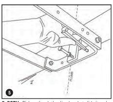
**5. BOTH:** Pick up the clothesline bracket slide it under the 'MTA'. Line up the centre clothesline bracket hole with the 'MTA', using it as a template, mark the remaining side holes through the bracket onto the  $2^{\circ}$  offset line then remove the bracket.
