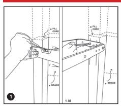
**1.** Mark height location approx 185cm from ground level & use a spirit level to draw a horizontal line for both brackets that is slightly offset by 2° with an inward tilt to each other (the spirit level bubble will be uncentered). Draw vertical lines through the horizontal line marking the desired bracket positions by picking up the bracket and marking through at least 2 bracket holes for structural rigidity or 3 holes for wider posts.
