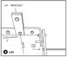
**8. INSTALLING 2ND BRACKET:** Repeat fixing process as per L/H bracket. **R/H bracket location** - feed cable through L/H bracket's 1st hole closest to wall pulling along wall & mark at the end of the cable. This is the centre hole location maximum distance of the R/H bracket.
