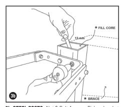
**3b. STEEL POSTS:** Nut & Bolt Access - Pick up bracket & place washers on hex bolts through the bracket and into the post placing a washer and nyloc nut onto the thread inside the post by hand. Repeat with all hex bolts, washers & nuts. Use 13mm spanner & ratchet to tighten all hex bolts to 95%.
