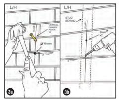
**3a. BRICK:** Now hammer drill with 10mm masonry bit both marked/cross holes to a depth of 75mm. Remove dust & debris & hammer in 2 orange plugs until flush with wall ready for the 75mm bolts.
