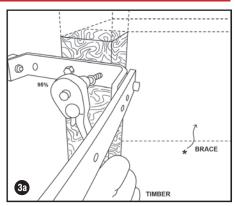
**3a. TIMBER POSTS:** Place washers on coach bolts & use the spanner to fix 'all coach bolts & washers' into the drilled holes to 95% tightness.
