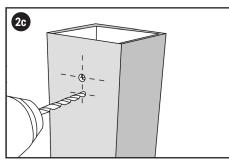
**2c. POST STEEL: Nut & Bolt for rear access:** Drill holes on marked locations through the post skin using the 6mm drill bit.
