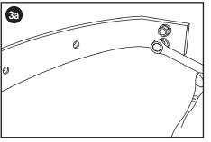
**3a. BRICK/STUD/TIMBER POST:** Pick up 1st coach screw provided, slide washer on & by hand fasten screw through bracket to 95% tension then repeat for 2nd fastener & hole. Now tighten to 100% for both screws. Do not over tighten but keep screws snug & tight.
