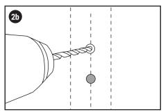
**2b. STUD/TIMBER POST:** Find centre of first stud location or post. NOTE: STUDS - BEFORE DRILLING find 2nd stud location within cable length provided. Drill holes using a 5mm drill bit to a depth of 70mm.
