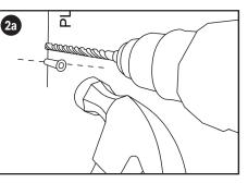
**2a. BRICK:** Place bracket down & drill into marked holes to 70mm depth using the 8mm masonry drill bit. Blow dust & debris out of hole & insert plastic plugs provided & hammer in flush.
