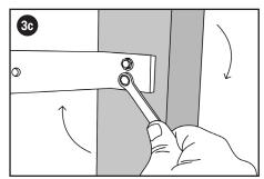
**3c. POST STEEL: Tapping for no rear access:** Place washer on screw & put through the bracket hole. Whilst keeping square turn in by hand followed by a 10mm spanner & tighten to 95%. Then repeat for 2nd hole & tighten to 100% on both screws- snug to finish- do not over tighten.
